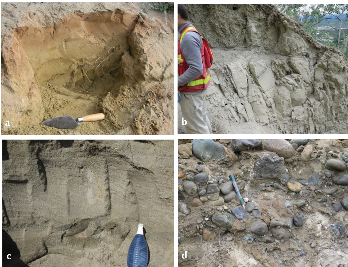
Figure 20. Field photos of selected samples analysed for grain size distribution in Figure 19: (a) loess unit of sample MAB 06-23-02-01; (b) laminated silty clay of sample MAB 09-17-02-01; (c) medium cross-bedded sand of sample MAB 09-17-01-03; and (d) sandy gravel of sample MAB 09-16-01-05.
