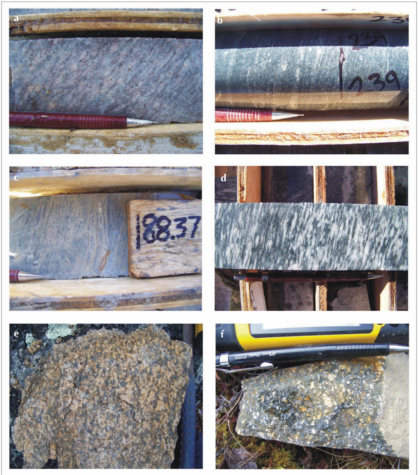
Figure 3. Photographs of Coffee property area rock units: (a) augen gneiss (CFD033 – 167.3 m); (b) biotite-feldspar schist (CFD067 – 239 m); (c) feldspar-quartz mylonite (CFD038 – 188.3 m); (d) mylonitized gabbro (CFD060 – 145 m); (e) granite (outcrop; Kona area); and (f) andesite porphyry (sampled from trench in the Supremo area).
