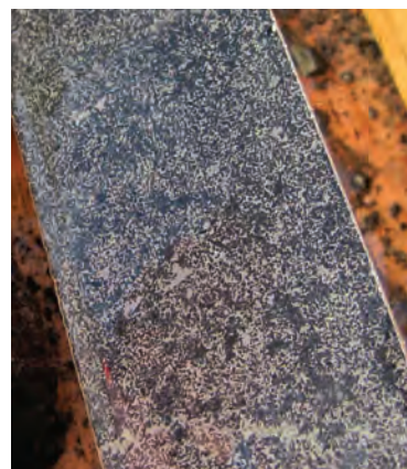
Figure 29. Net-textured sulphides in core at the Wellgreen property of Prophecy Platinum Corp.
