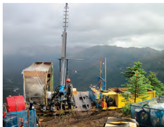
Figure 11. Diamond drilling at Northern Tiger's 3Ace gold property.
