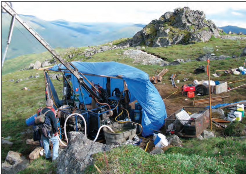
Figure 27. Diamond drilling at the White River property optioned by Driven Capital Corp.
