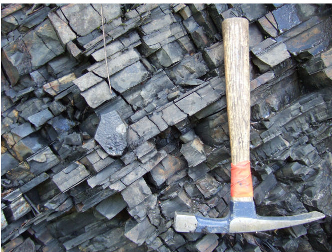
Figure 9. Siliceous silty mudstone and shale outcrop. Mudstone is resistant and forms >90% of unit. The silty mudstone weathers into blocks with semi-conchoidal fracture. Shale is observed as thin partings (<1 cm) between mudstone beds.
