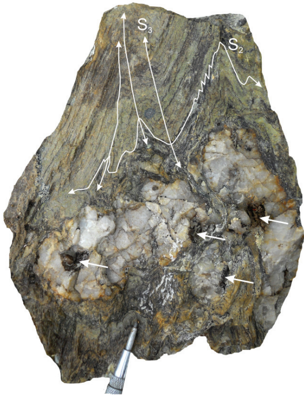
Figure 2. Sample of Klondike schist, showing an F_3 fold with an accumulation of quartz and calcite in the hinge zone. Clots of partially leached calcite are indicated by the white arrows. Quartz and calcite are interpreted to have migrated into low-strain fold hinges during D_3 deformation, potentially from pre-existing, D_2 -generation segregations.
