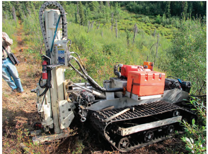
Figure 13. Groundtruth Exploration's Geoprobe on the King Solomon Dome property. The Geoprobe is a direct-push, track-mounted drilling machine. It can obtain soil samples and samples from the overburden/bedrock interface.
