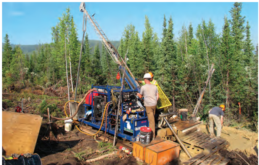
Figure 15. Diamond drilling at Metals Creek’s previously undrilled Squid East property.
