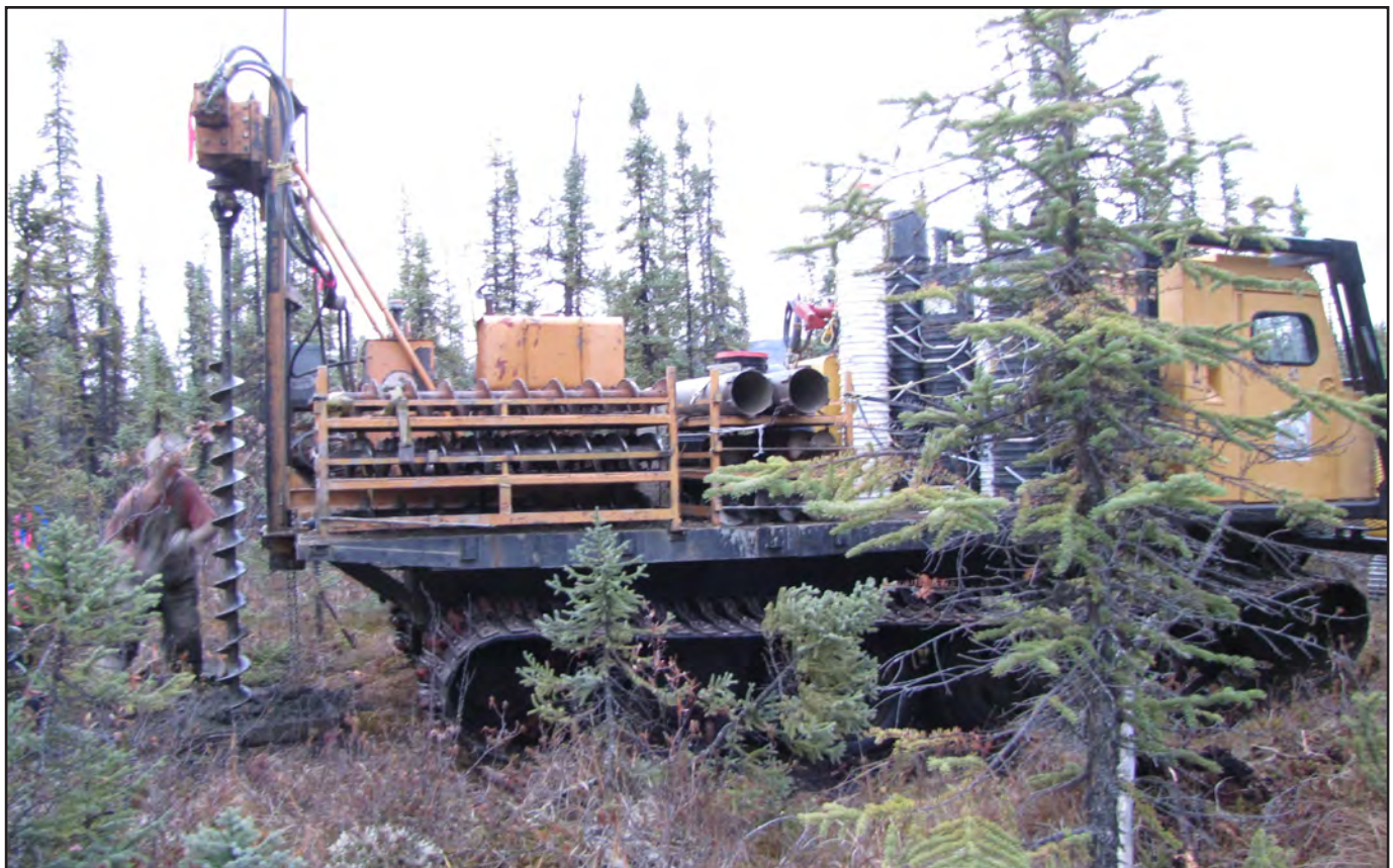
View of the 8" auger drill and Nodwell used for testing Goodman Creek.
