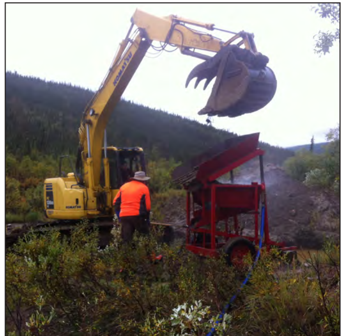
Using a Komatsu 138 and a small test plant to prospect Bell Creek.
