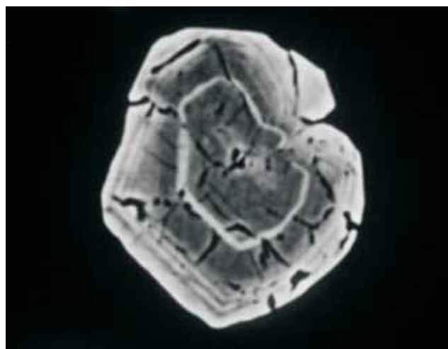
Figure 10. Bands of high As content (light coloured) within a fine, rounded grain of pyrite approximately 30 microns in size from the Supremo zone.
