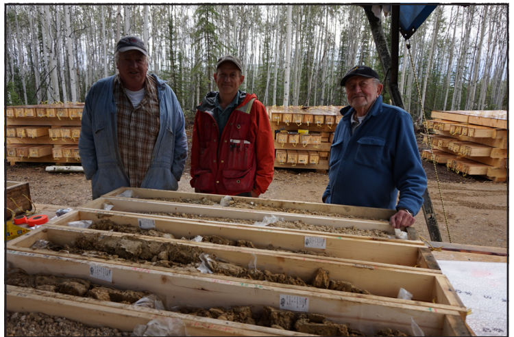
Figure 12. Dave Johnson, Bill LeBarge and Rod Hunt (L to R) of Wolfhead Mining and Discovery sample and describe the stratigraphic units contained within their sonic drill core.
