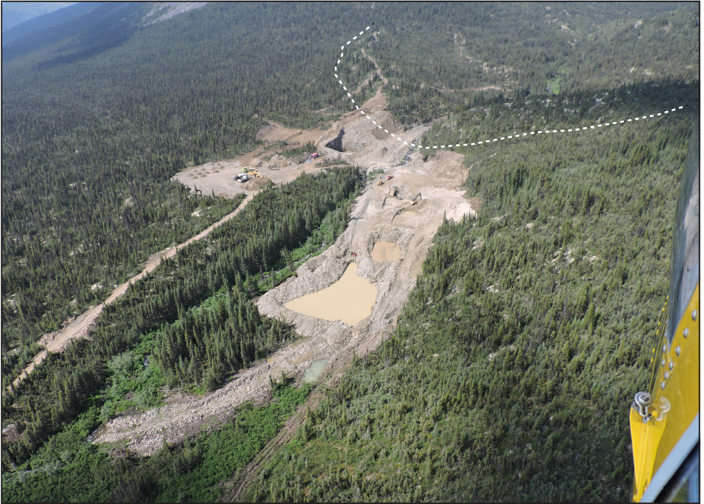
Figure 9. An aerial view to the west of Granite Creek in the Gustavus Range near Keno City. Mining is focused immediately downstream of an end moraine deposited from an alpine glacier during the McConnell glaciation (dashed line marks the base of the moraine ridge). The deposit consists of outwash gravel derived from reworking the end moraine and recessional moraines farther up-valley. Photo courtesy of William Leary.
