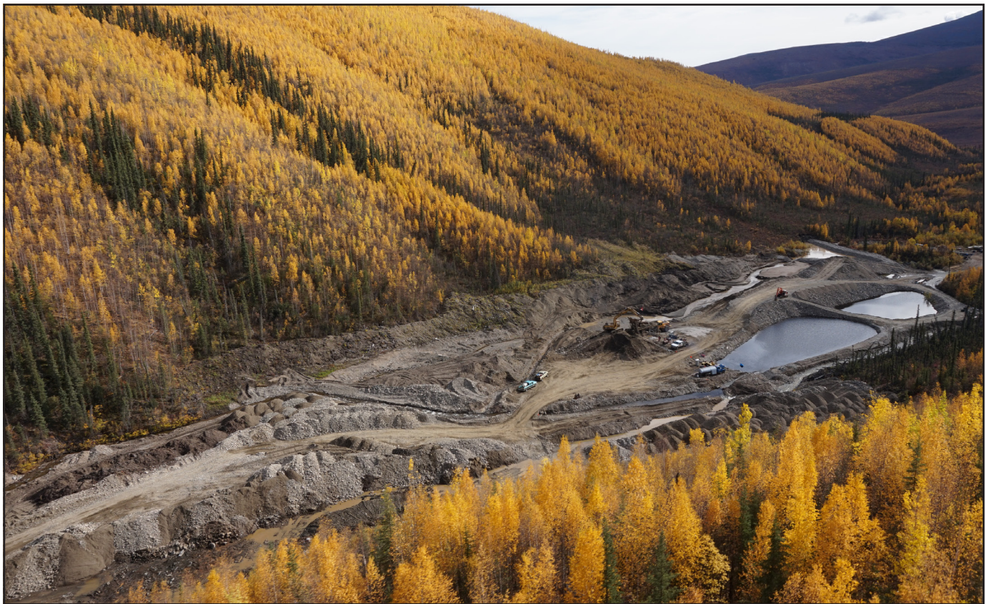
Figure 8. An aerial view to the southeast over P. Joseph's operation on Cheryl Creek. The placer gold is contained within a boulder-rich gravel containing magnetite. In general, the right-limit of the creek contains more gold than the left-limit in this area of the valley.
