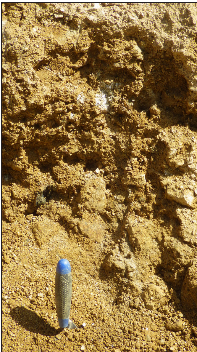
Figure 6. Pre-glacial gravel (Unit 2) exposed in lower Back Creek. Gravel is pervasively weathered and iron-stained. Clasts are variable in lithology but local in source.
