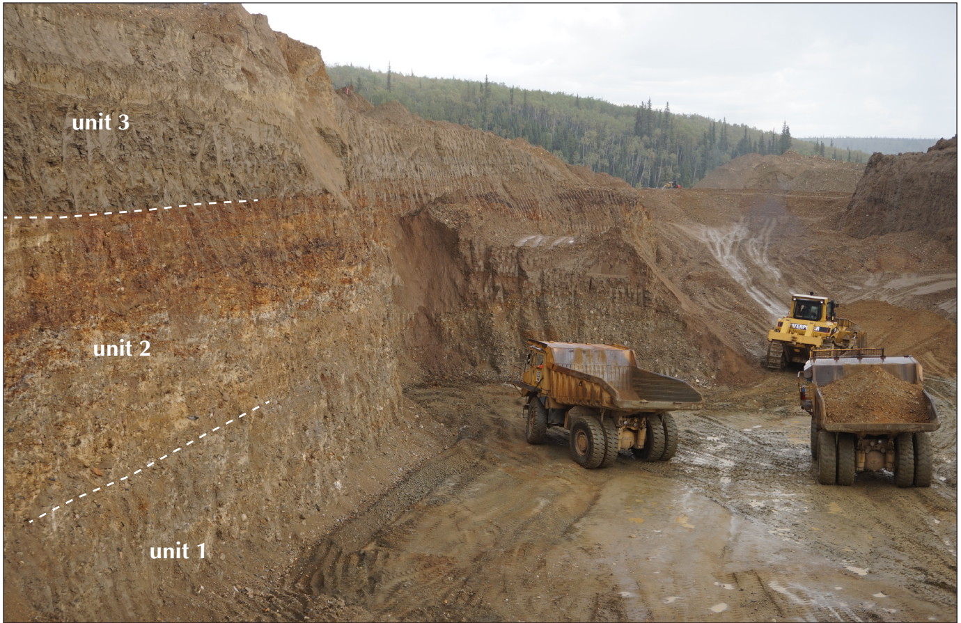
Figure 10. Dulac Mining’s cut on the left limit bench of All Gold Creek. Units 1 and 2 represent the Pliocene gravel that is equivalent in age to the upper White Channel Gravel. Unit 3 is a glacial lake sediment that was deposited during one of the first glaciations to block drainage in the Tintina Trench. The oxidized horizon at the top of unit 2 is the former pre-glacial soil about 2.6 million years old.
