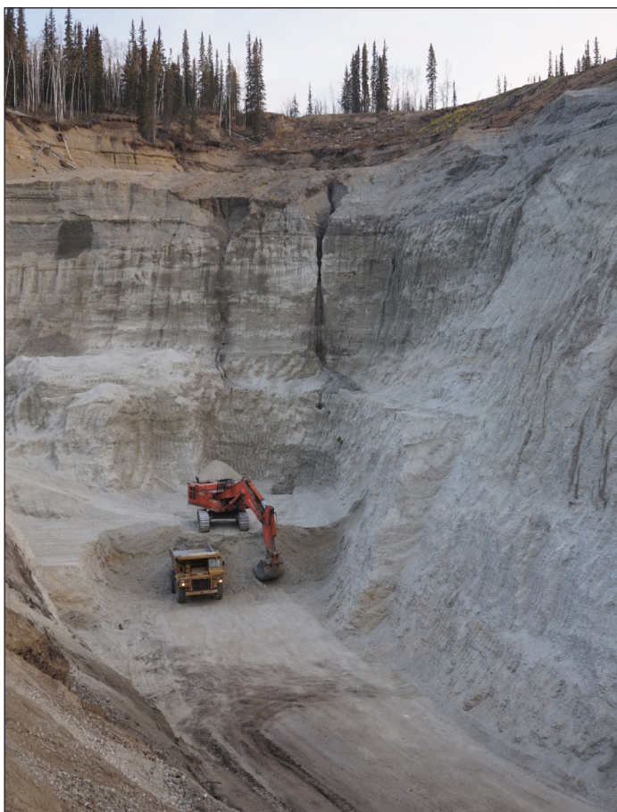
Figure 9. A view to the north of Northern Shoveler's cut on Lovett Hill in late September, 2016. Much of the season was spent excavating to the high grade pay channel on bedrock.
