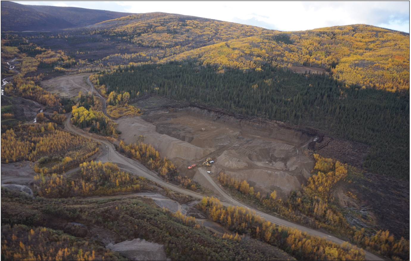
Figure 5. A view to the southwest of Fine Gold Resources left limit bench cut in 2016. Bulldozers are used to remove overburden and expose the pay gravel. The channel continues upstream in this photo and is visible by the change in slope at the base of the hill.
