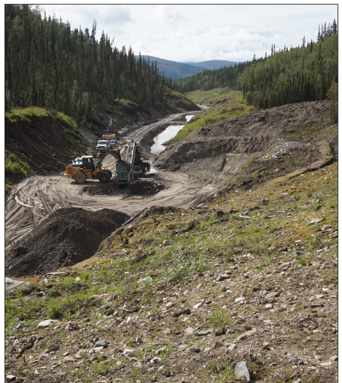
Figure 4. Lori Cail's wash plant and settling ponds on upper Canyon Creek. Mining can be challenging in narrow valley settings but Mr. Cail does an excellent job managing water quality and recontouring overburden so vegetation can re-establish.
