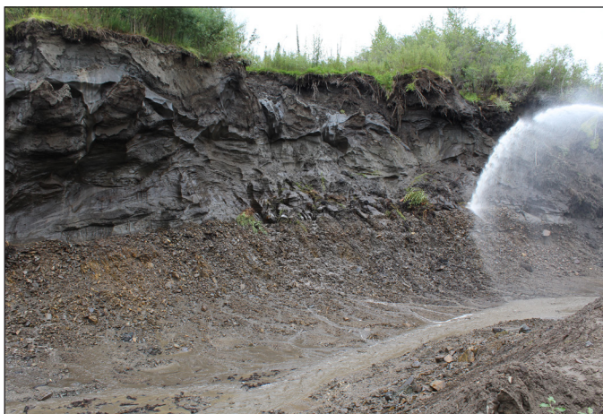
Figure 12. Exposure of the left limit bank at Rod Smith's mine on upper Black Hills Creek. The pay gravel is overlain by 20 m of ice-rich muck and a monitor is used for stripping.
