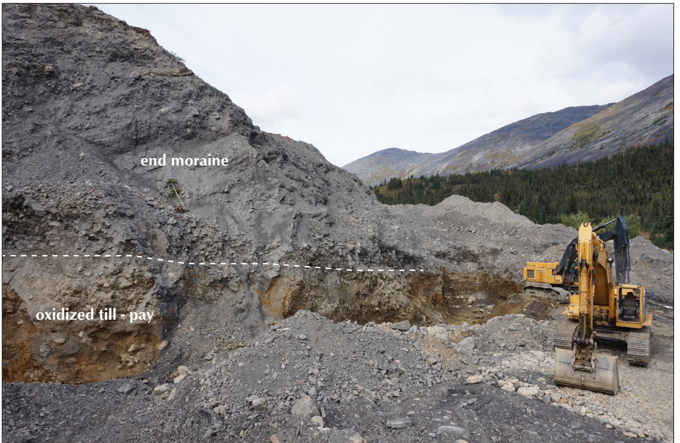
Figure 19. Jim Davies is mining oxidized (orange) till from under grey morainal sediment deposited during the last glaciation. The oxidized-gold-bearing till is likely from an older alpine glacier that reworked a pre-existing fluvial deposit.
