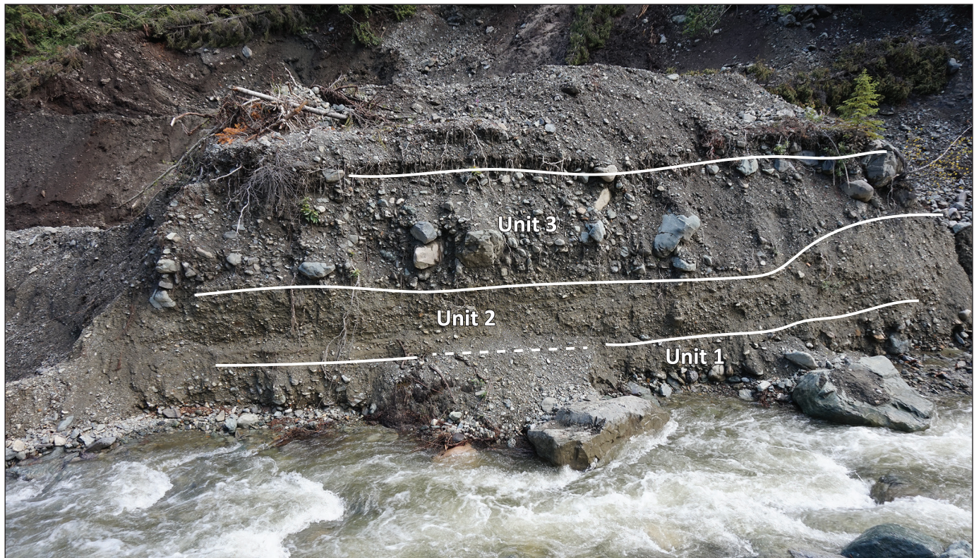
Figure 5. Stratigraphy of a right-limit cut at Russel Nelson's Arch Creek placer mine in 2016. Unit 3 in photo is approximately 1.5 m thick.
