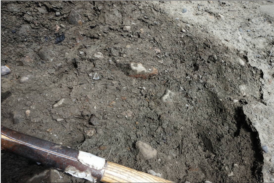
Figure 13. Unit 8 at Site 2 is a compact glacial diamict with a clay-silt-sand matrix. Shovel handle is 5 cm wide.
