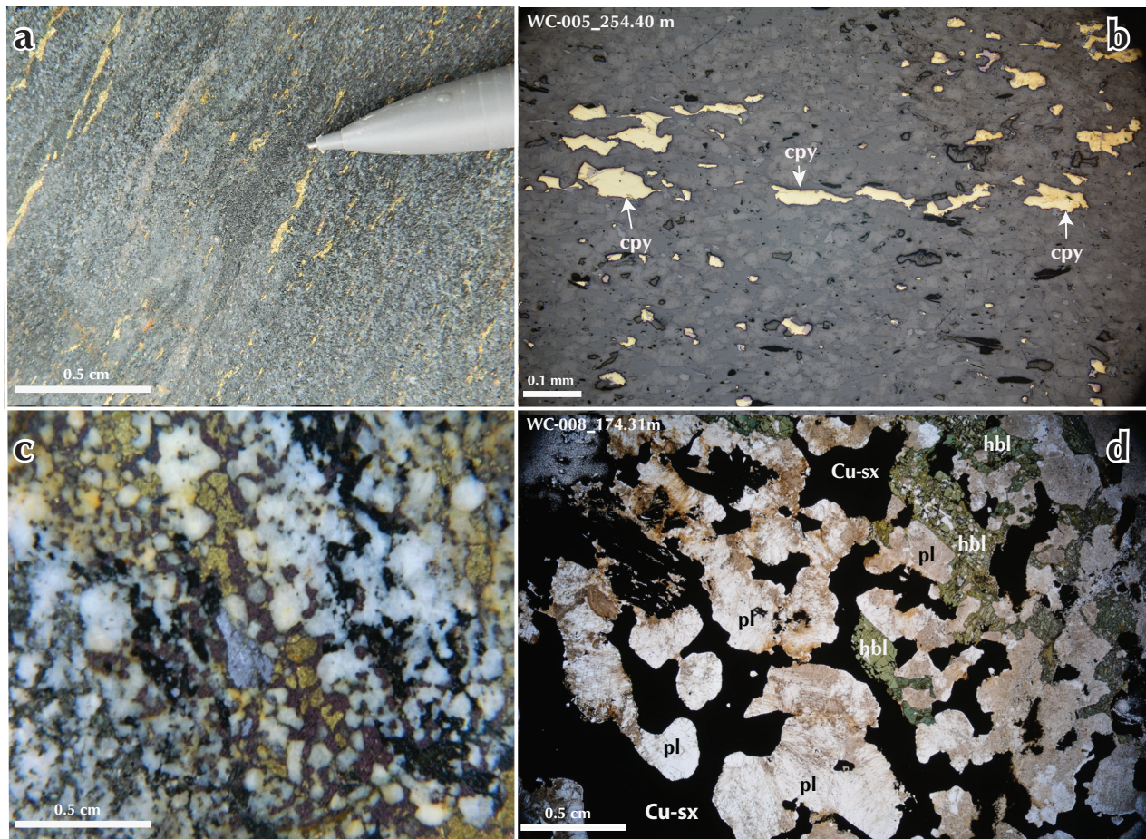
Figure 11. Hypogene mineralization features: (a) foliation-parallel chalcopyrite stringers in feldspar-amphibole schist; (b) net-textured copper sulphides in migmatitic host rocks; (c) reflected light photomicrograph of foliation-parallel blebs and stringers of chalcopyrite in feldspar-amphibole schist; and (d) transmitted light photomicrograph of net-textured copper sulphides in migmatite host rocks (plane-polarized light). pl=plagioclase; hbl=hornblende; and Cu-sx=copper sulphide phase.
