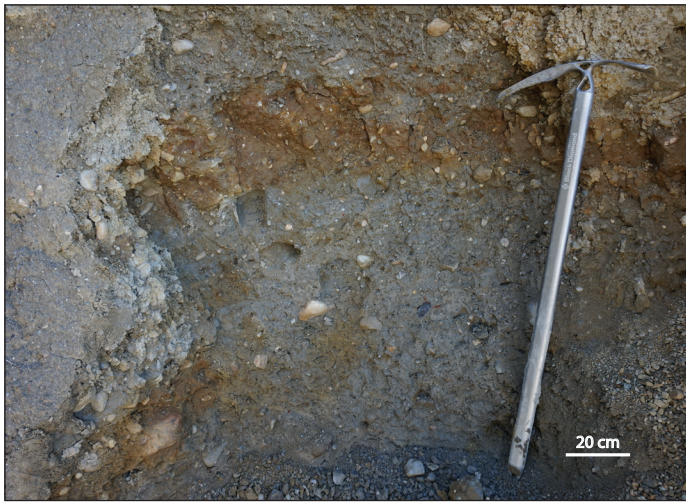
Figure 10. Typical appearance of Till B. It is a compact, medium-grey-brown, silty-sandy cobble diamict with weak stratification. Reddish brown/rusty sand lenses occur throughout the unit and are considerably more cemented than surrounding matrix.
