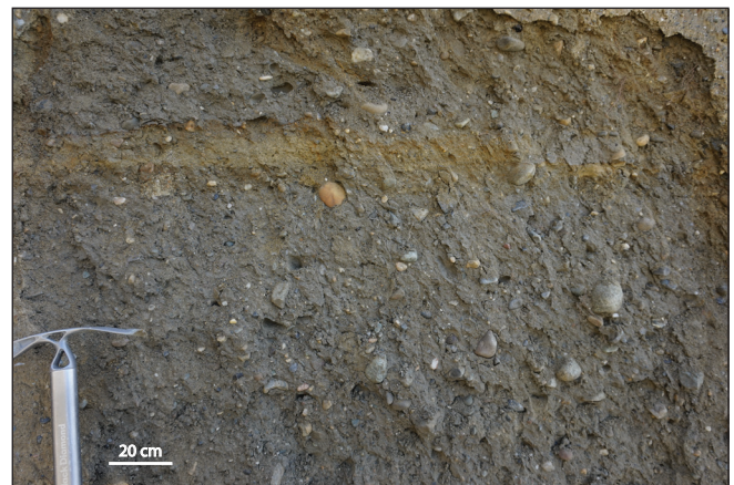
Figure 12. Typical appearance of Till A. It is a compact medium-brown, silty-sandy cobble diamict. Abundant quartz, quartzite and granite pebbles in the unit are well-rounded, and many granitic pebbles are highly weathered.
