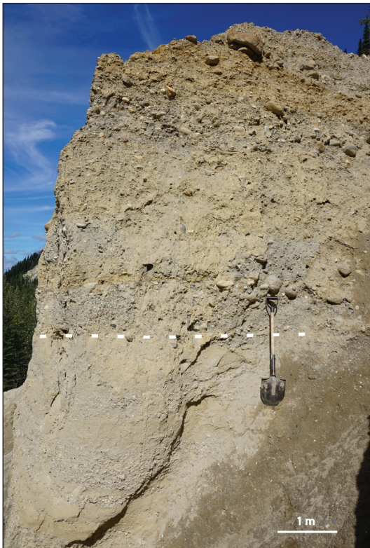
Figure 13. Lower contact between inferred Tertiary sediments and Till A (marked with dashed line). It is heavily oxidized, horizontal, slightly undulating, and sharp.
