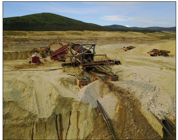
Figure 4. Schmidt Mining's wash plant on the Quartz Creek bench with the right limit Pliocene section exposed in the background. The wash plant is capable of processing 200 loose yd 3 per hour.
