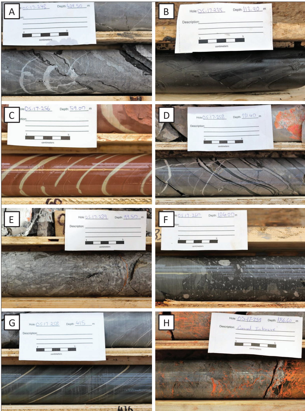
Figure 5. Representative rock samples from the Osiris cluster from oldest to youngest: (A) C-LST1; (B) C-SLC; (C) O-MST1; (D) O-LST1; (E) O-DST with typical debrite textures; (F) O-DMT; (G) O-LST2; and (H) C-INT.
