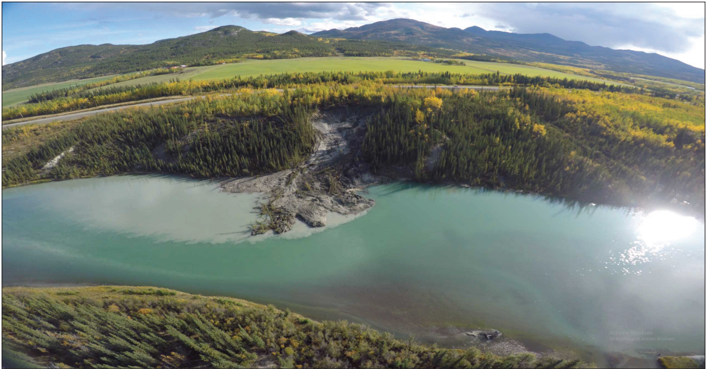
Figure 8. Drone photograph of a thaw slump along the Takhini River west of Whitehorse. View looking southward.
