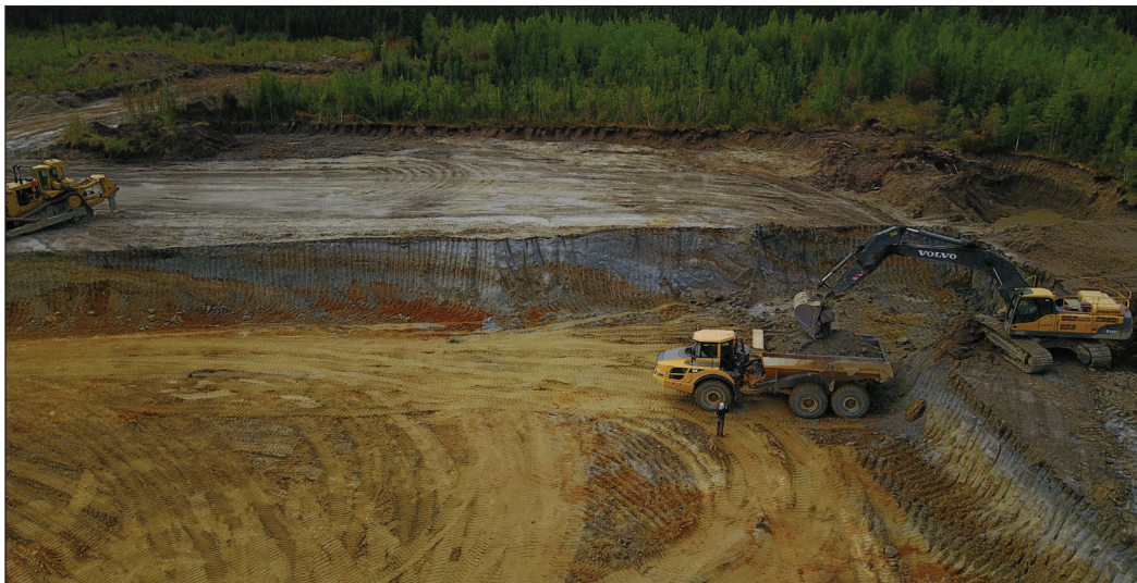
Figure 7. A view of the Paradise Hill cut showing a thin layer of White Channel gravel overlying the orange oxidized Paradise gravel. Virtually no muck overburden is present at this location.
