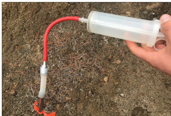
Figure 7. Soil gas extraction using 150 ml syringe. Red rubber tube connects directly to valve on ionization chamber. Probe flagged with orange tape.
