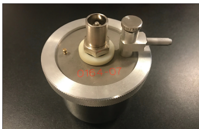
Figure 8. IK-250 ionization chamber for radon concentration measurement, 250 ml capacity. Serial number is red, electrodes are brass pin at left and in central cylinder. Valve at right (knob above protruding tube).
