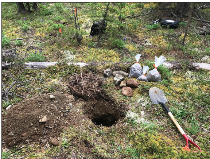
Figure 6. Photograph of sampling site 20MK-010 on June 18, 2020. Glaciofluvial gravel overlying Mandanna member of the Aksala Formation (sandstone and conglomerate). Three bags of sediment, from left to right, for clast lithology/geochemical analysis, matrix geochemistry, and grain size distribution. The spectrometer case is visible in top right and a probe flagged with orange tape can be seen in the top left.
