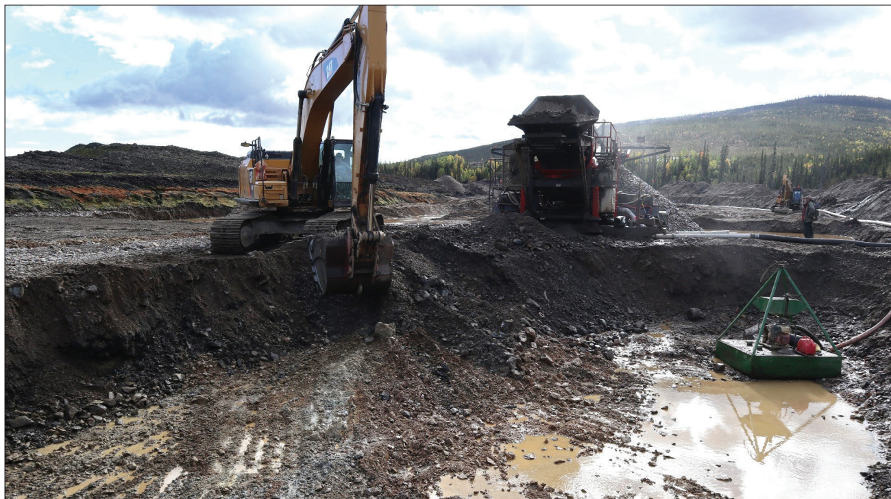
Figure 12. A view of M2 Gold Mines' plant on the Sixtymile River. Their mobile trommel plant reduces costs associated with hauling pay gravel.
