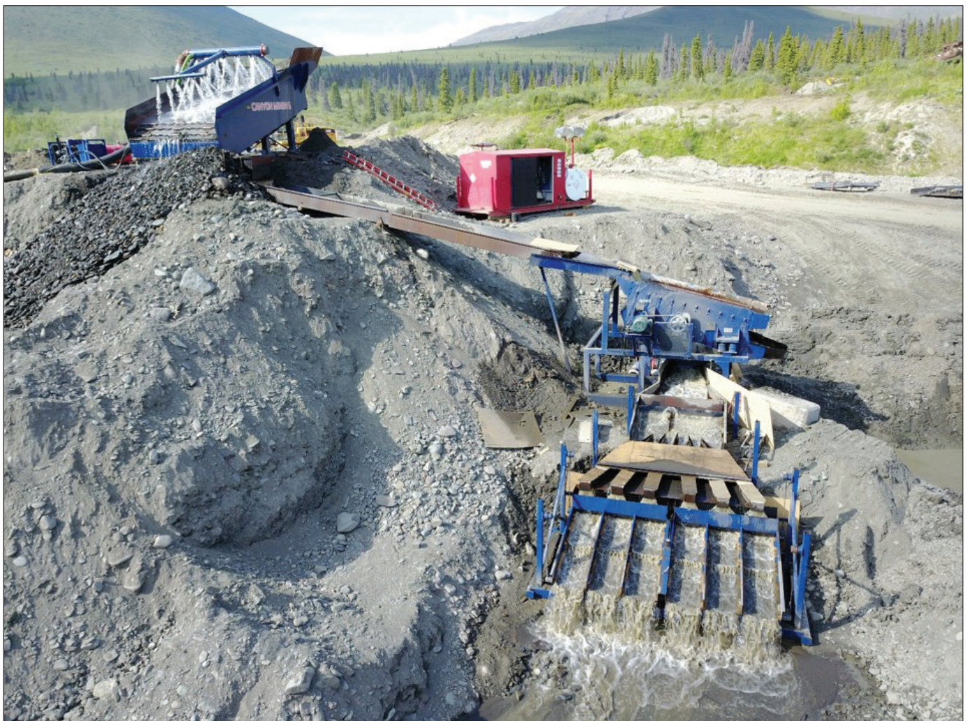
Figure 22. Canyon Mining Limited's wash plant and sluicing configuration on Fourth of July Creek.
