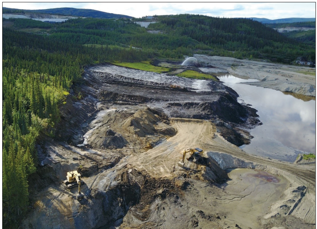
Figure 9. A view to the north looking down the left limit of Hunker Creek near the mouth of Last Chance Creek. The excavators are sitting on a low-level bench, which was the target of operations for the Sailer mine in 2020.
