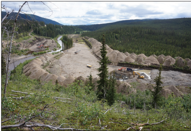
Figure 3. A view looking up the Indian River over Slate River Mining's operation. Overburden is strategically stacked adjacent to the cut minimizing transport distances and facilitating reclamation.
