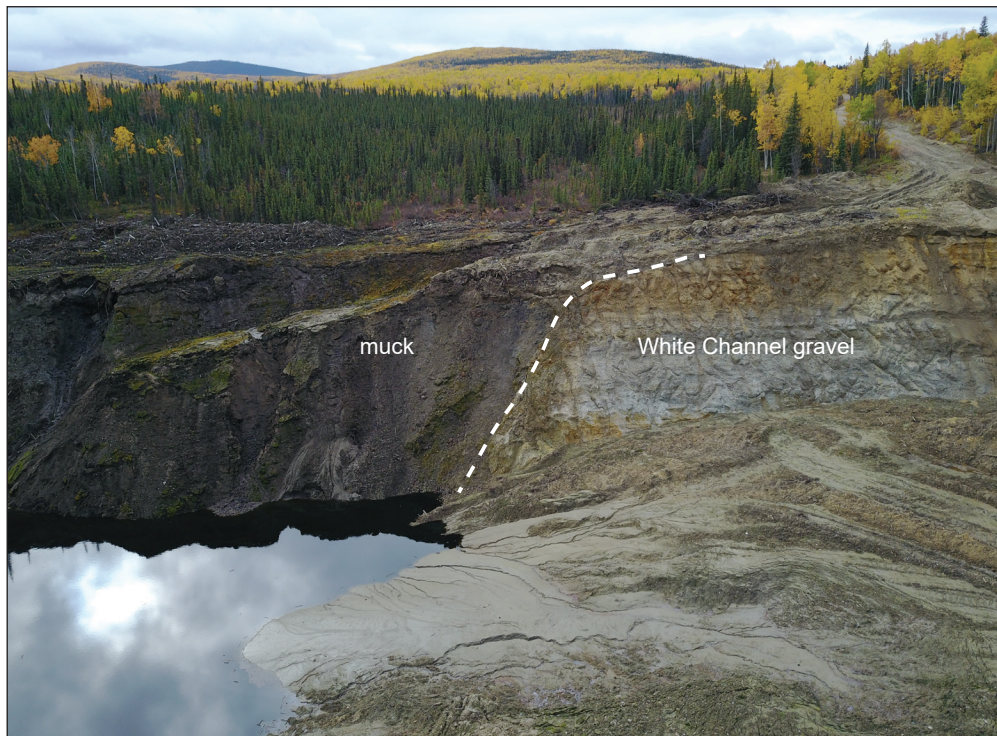
Figure 4. Fine Gold Resources cut in 2021 where they exposed a White Channel terrace on the left limit of Indian River.
