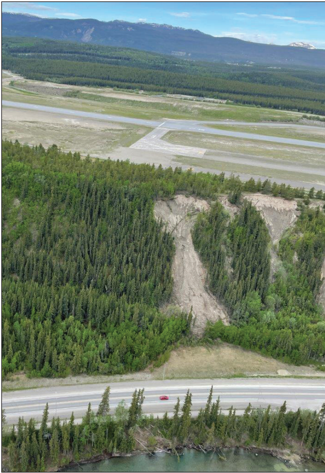
Figure 7. Aerial photo of a June 2021 landslide documented by Lipovsky on the scarp below Whitehorse Airport. View looking west; Robert Service Road in the foreground.
