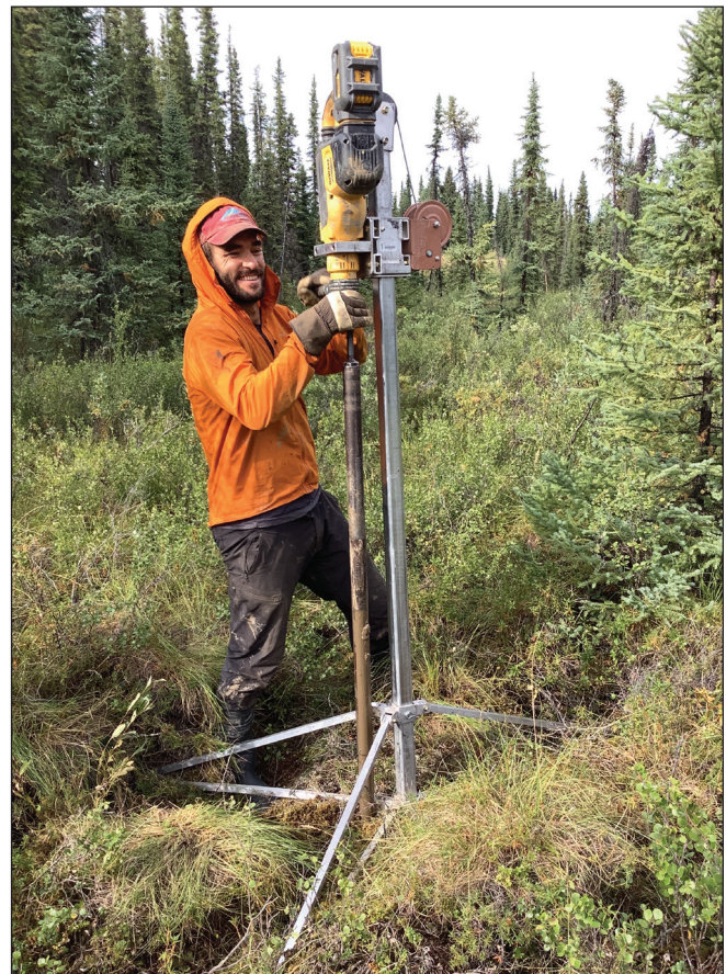
Figure 8. Derek Cronmiller drilling a borehole near Beaver Creek. The borehole was instrumented with a thermistor and is part of YGS’ network of permafrost monitoring stations.
