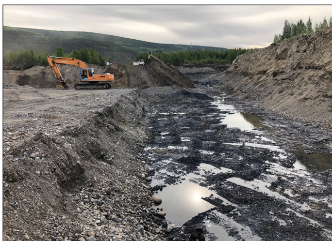
Figure 9. Slonski and Elgie's cut on the left limit of the Klondike River valley. The stratigraphy consists of Klondike River gravel overlain by sand derived from Hunker Creek.
