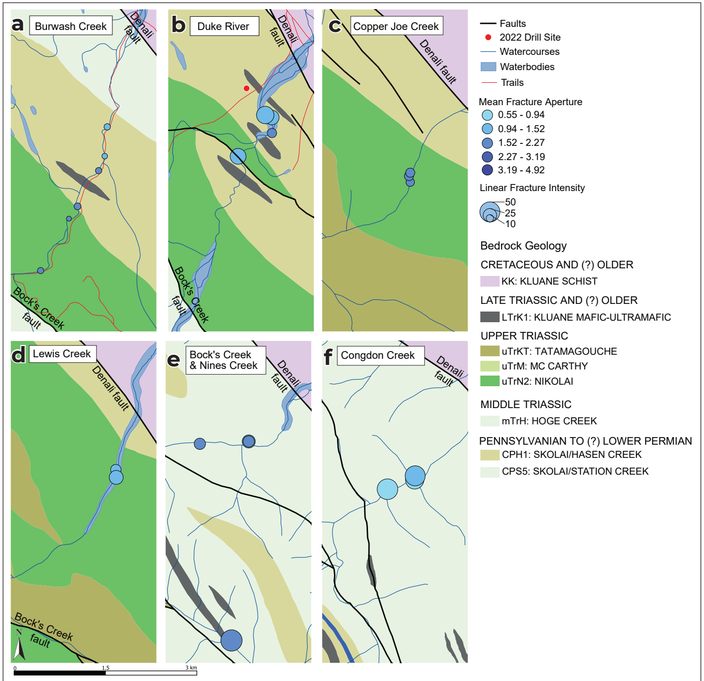
Figure 10. Linear fracture intensity per scanline collected on foot at outcrops located along creeks. These indicate the proximity of each outcrop to faults in addition to the Denali fault. These include the Bock's Creek and unnamed faults.
