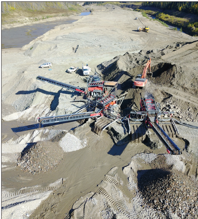
Figure 11. Three wash plants being fed by a Hitachi 470 excavator at H.C. Mining Ltd. operation on Henderson Creek.
