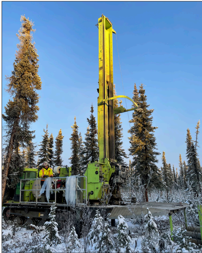
Figure 2. Northern Sonic Drilling and Consulting’s sonic drill at site YGS_BeaverCreek_BH4 in Beaver Creek.
