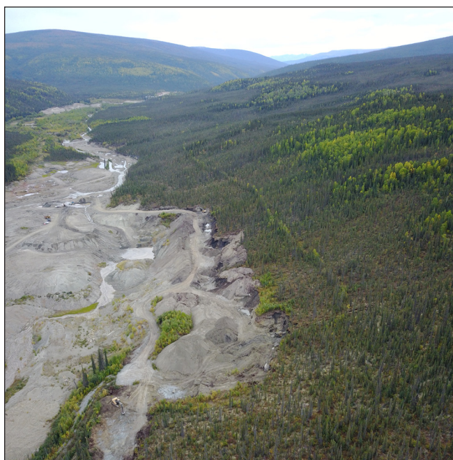
Figure 14. Rally! Mining ULC's buried left limit bench on Duncan Creek. The view is looking upstream at a large cut that was completed to evaluate the deposit.
