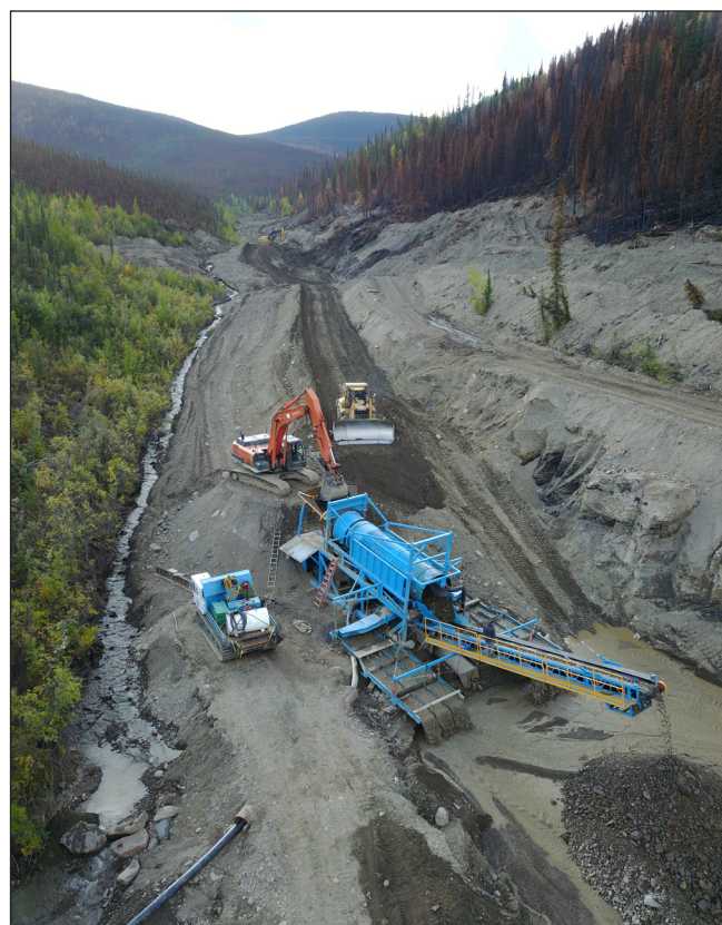
Figure 15. L. Andre's operation on 15 Pup, and his newly fabricated trommel actively sluicing pay.
