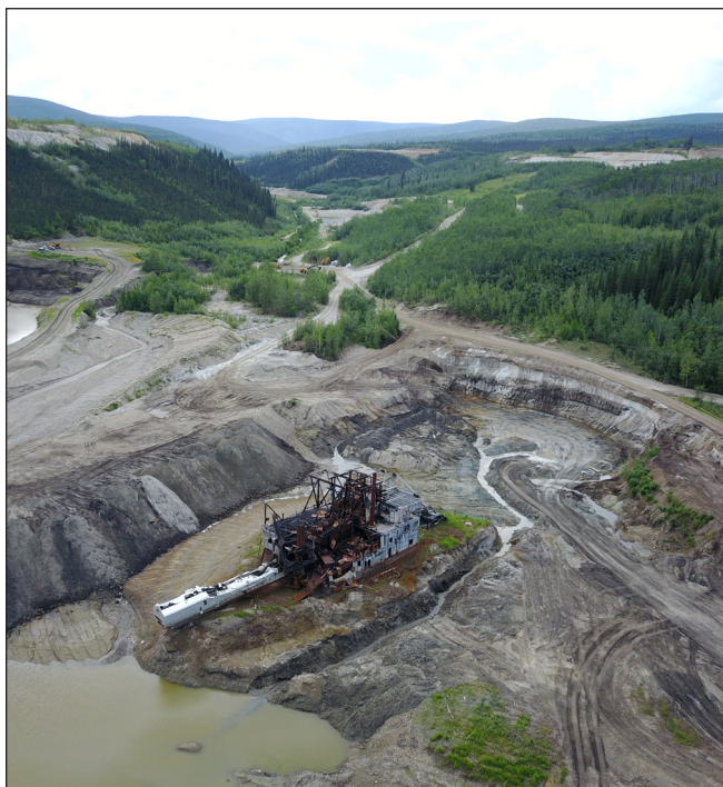
Figure 6. Dredge 11 at the mouth of Last Chance Creek; Tatra Ventures Ltd.'s cut is exposed behind the dredge.
