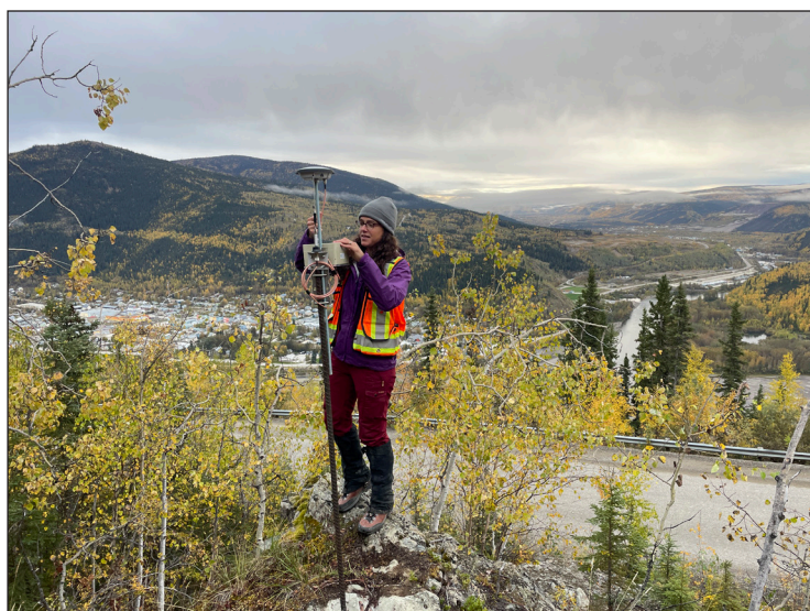
Figure 6. Panya Lipovsky adjusting a GPS unit installed on the Sunnydale landslide.
