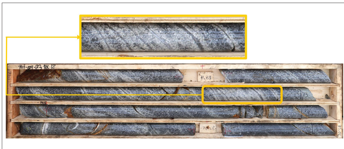
Figure 8. Sheeted quartz-sulphide veins with wide sericitic halos from drillhole HIT-004 at Rackla Metal's HIT property; close-up photograph is from the inset outlined in yellow (Rackla Metals Inc., 2023b).
